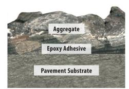
SafeLane® CA-48 surface overlay is a proprietary compilation of a special aggregate and epoxy that retain and release deicing agents as determined by weather conditions. Additionally, this aggregate component supplies increased friction year-round unlike automated anti-icing spray technologies
