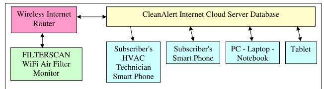
**FILTERSCAN** status is sent to the database periodically and can be sent upon demand from the **FILTERSCAN** by depressing the SEND button. Status includes percentage of air filter life used, battery condition, system error, time since last filter service, and software version. Software updates can be performed remotely from the database to each individual **FILTERSCAN** *WiFi* Air Filter Monitor.
