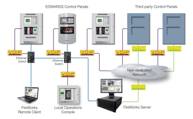
Enterprise Level Management and Control: EDWARDS provides the system and point capacities along with network solutions from Cisco to provide enterprise-level communications and IP point control and monitoring worldwide to protect and manage critical cloud-based facilities.
