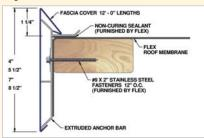
Fully Adhered or Mechanically Attached Single-Ply Version
