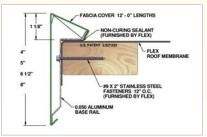
Fully Adhered or Mechanically Attached Single-Ply Version
