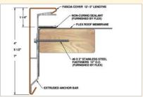
Fully Adhered or Mechanically Attached Single-Ply Version
