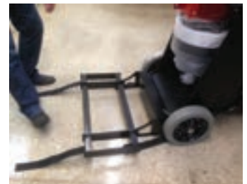
Lift back end and move vac trailer into position to hook on front of vacuum.
