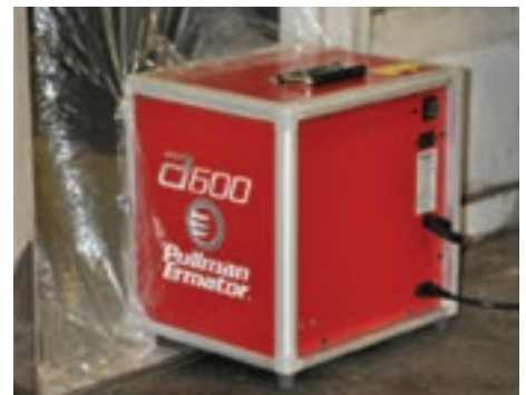
A-600 air scrubber in use on a job site.
