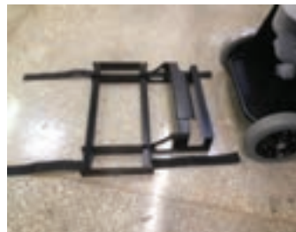
Lay vac trailer on floor with small end facing vacuum. Undo velcro straps.
