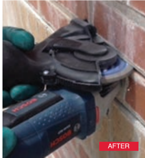
Dust hood captures harmful construction dust.
