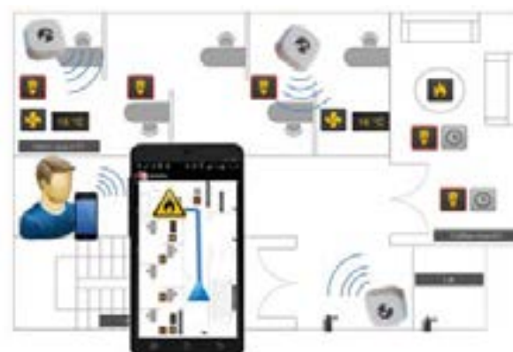
PcVue Solutions Mobile app automatically adjusts the display of information depending on the identity of the user and its position
