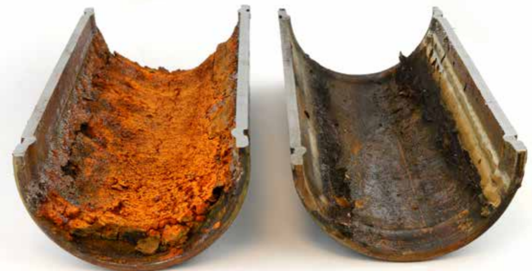
20 Month Pipe Test with Air
