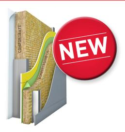
ROXUL® COMFORTBOARD™ CIS (Commercial Insulated Sheathing) is a rigid, high density, non-combustible, stone wool insulation board designed for use as an exterior continuous insulation in commercial applications. This thermally efficient, moisture resistant, vapor permeable board is effective against fire, moisture thermal bridging and allows for superior drying potential.
