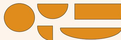
Duct profiles - the most common profiles are round and half round ducts, which are supplied as standard solutions. Other solutions require custom design at FabricAir®.
