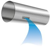
A conventional duct with grills or diffusers distributes the air at certain points, resulting in uneven air distribution.
