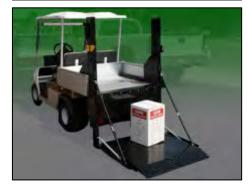
Weight Capacity: 800 lbs. max Control: Constant pressure up/down switch Key lock on control switch Engineered and designed for industrial and commercial use Available for most electric carts and trucks ! Year Limited Warranty
