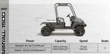
Features our foolproof IntelliTrak<sup>™</sup> fully automatic four-wheel drive system as well as our semi-independent four-link rear suspension system for a smooth ride, even when fully loaded.
