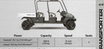
With Club Car's exclusive IntelliTrak<sup>™</sup> automatic four-wheel drive system and four forward-facing seats, this vehicle carries 4 passengers and their gear over the roughest terrain.
