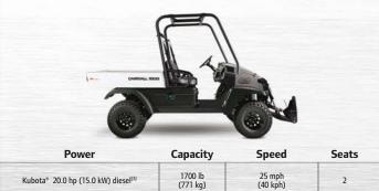
Features both our foolproof IntelliTrak<sup>™</sup> fully automatic four-wheel drive system and our IntelliTach<sup>™</sup> fully hydraulic attachment system with three attachment tools. The definition of versatility.
