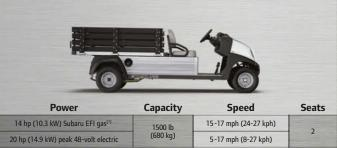
A nearly 6 foot (67.6 in/171.7cm) long bed makes transporting cargo easy and efficient, yet independent suspension and rack-and-pinion steering deliver a smooth ride.
